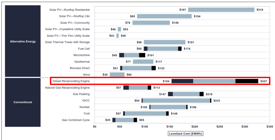
Figure 5.18 LCoE comparison of different alternative and conventional power generating technologies operating in the US with sensitivity to fuel prices: dark areas correspond to \pm 25\% fuel price fluctuation [27]
