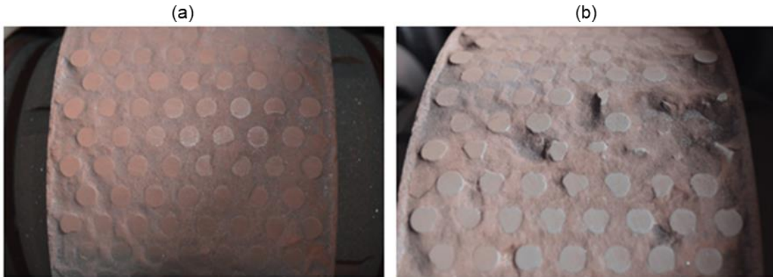
Figure 3.5. Difference between two rotating rolls in a lab-scale HPGR used to process iron ore concentrates with different wear patterns. Figure 3.5a shows the roll at the beginning of roll lifetime, whereas Figure 3.5b shows the intense surface wear after several hours of testing. Studs on both rolls are made of tungsten carbide.
