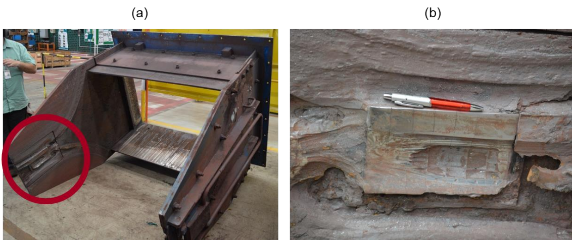
Figure 3.6. Cheek plate used in an industrial-scale HPGR (a) and the highlighted wear pattern of the same cheek plate (b). Cheek plate at the end of lifetime presented was registered for an HPGR pressing fine iron ore concentrates.
