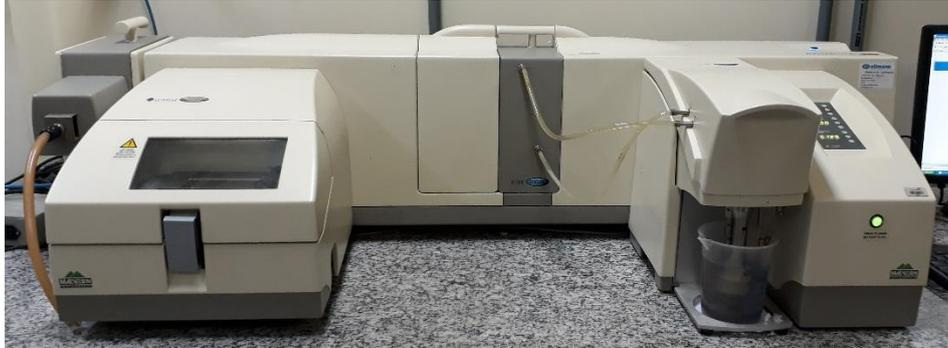
Figura 3.11: Granulômetro a laser Mastersizer 2000 Malvern Instruments
