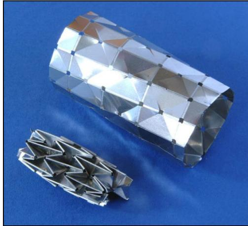
Figure 2-16: Stent graft developed with a Nitinol sheet, using waterbomb tessellation (Image credit: Kuribayashi, 2006).
