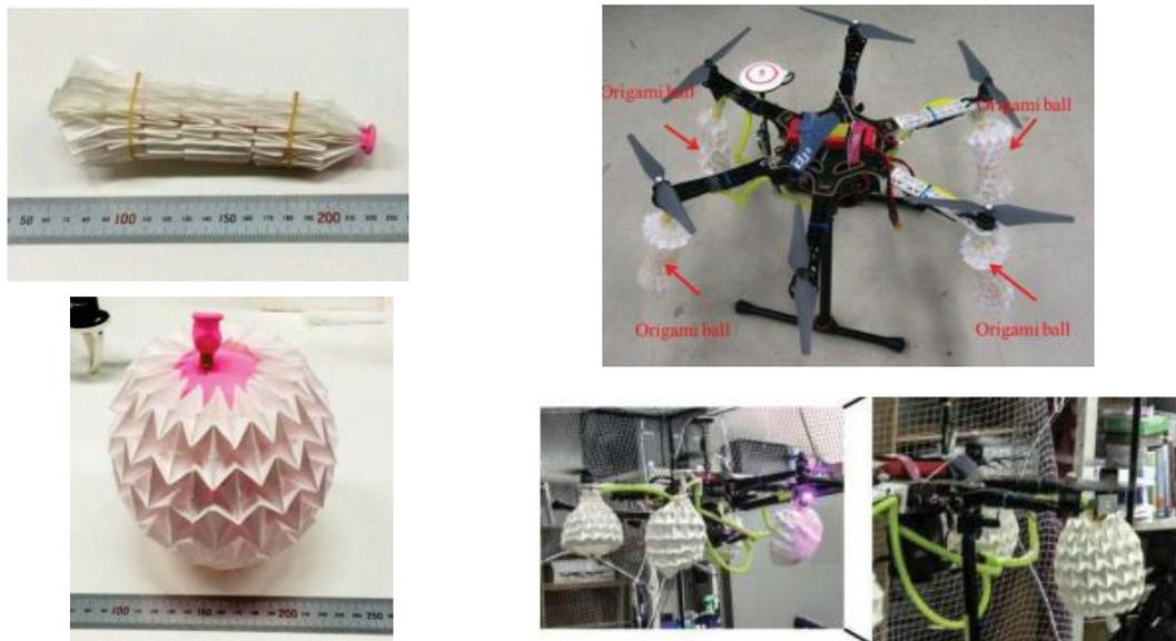
Figure 2-18: Application of a waterbomb tessellation as an inflatable drone landing gear for water landing (Image credit: Le *et al.*, 2014).
